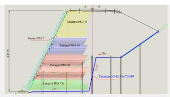
Typical cross section with decreasing tensile strengths depending on the height
