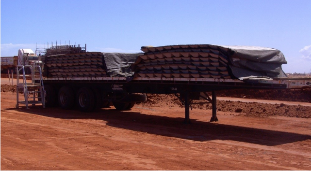
Transportation of the 2.6 m width flexible concrete mattresses
