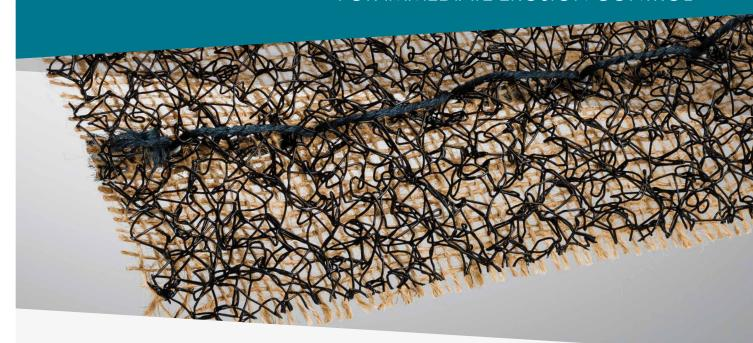
Enkamat J is a three dimensional polyamide mat with an open structure sewn to a biodegradable geotextile fabric. Enkamat J is used to prevent erosion on embankments, slopes and river banks.
