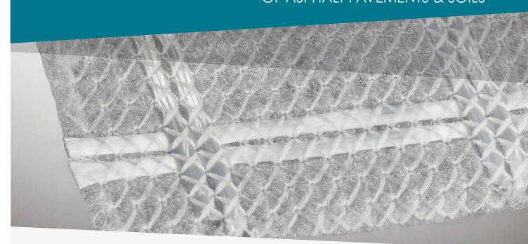
Enkagrid PLUS is a knitted geocomposite, comprising a geogrid made from high tenacity PVA or PET yarns combined with a nonwoven PET or PP geotextile. Enkagrid PLUS can be used for the reinforcement of asphalt pavements and soils.
