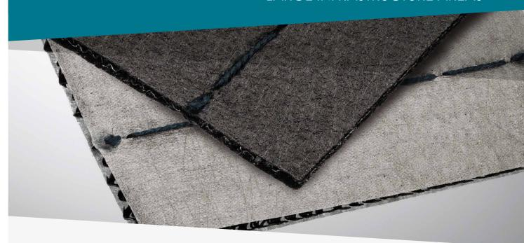
Enkadrain Wide consists of a 5 metre wide three dimensional monofilament drainage core with either a thermally bonded or needle punched nonwoven or woven fabric stitched to it. The product is a versatile and reliable geocomposite for landfills and large infrastructure projects.
