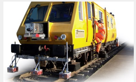
Typical Ground Penetration Radar device for railway lines
