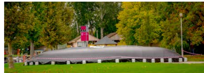
The two smaller tubes were pumped to a height of 2.3 m. The biggest tube is placed on top of the two smaller tubes.
