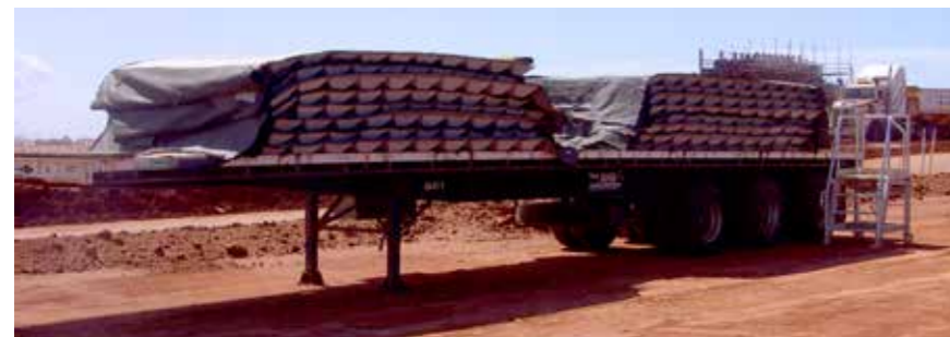
Transportation of the 2.6 m width flexible concrete mattresses
